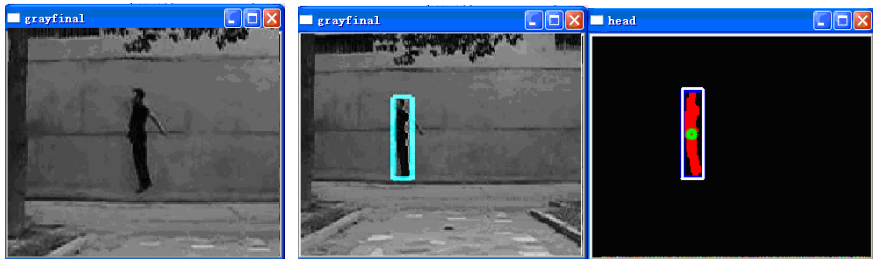
Fig. 5. Result of A Single Person. Both picture (a) and (b) show a side-jumping man, (a) is the result only use the silhouette contrasting, while (b) is the result of the new algorithm combining silhouette contrasting and centroid tracking. As we can see, the ameliorated arithmetic can recognize the suspicious action. The green point in picture (c) is the center of mass, and the write rectangle is the minimum one that includes the people’s silhouettes.
